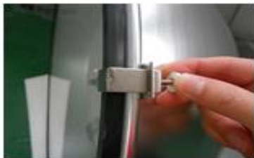
7. Screw in the safety clips
